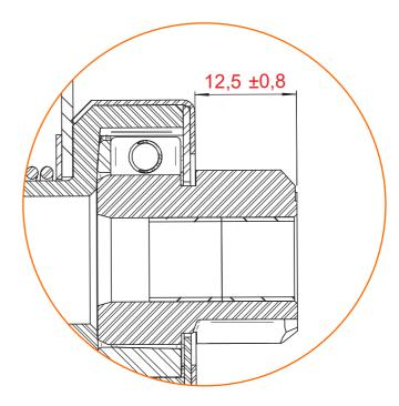
• If the 0328 is applied in the place of the 0294 it may cause damage to the starter drive and/or the vehicle's flywheel
