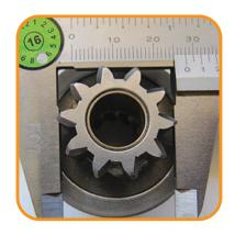
Align the **teeth horizontally** according to the red arrows and **support the upper teeth on the caliper ruler** as indicated in blue. **In this** way we have exactly the teeth's external diameter.
