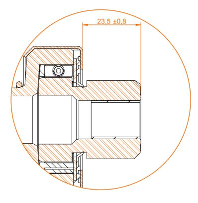
The 1194 has a higher gearing height (23.5) ± 0.8) and uses a rubber seal to prevent external contaminants (oil/dust/water/etc) from damaging the starter drive's internal system.
