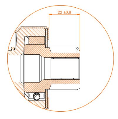
The 0629 has a lower gearing height (22  $\pm$  0.8)
