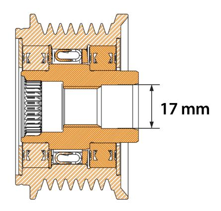
Be aware that the alternators on the market listed below will indicate the application of both pulleys. So, before purchasing, make sure of the rotor shaft diameter and consult the ZEN catalog.
